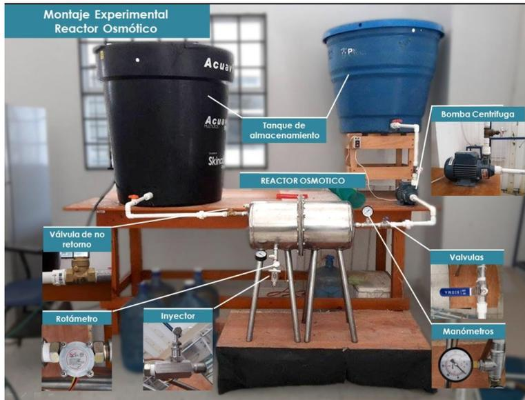
FIGURA 14 REACTOR OSMOTICO A ESCALA DE LABORATORIO
